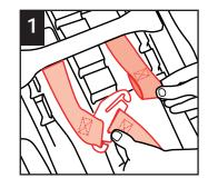
From the back of the seat, unfasten harness straps from splitter plate.
